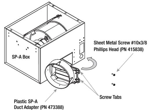
**3** Install screws provided to secure discharge.
