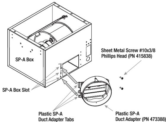
**2** Rotate plastic SP-A duct adapter (PN 473388) until the screw tabs meet SP-A box.
