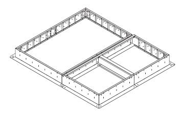
Greenheck VK-ERS curb is shipped in sections for field assembly. All required hardware is provided. Attachment to roof or structural members and building weather protection by others.
