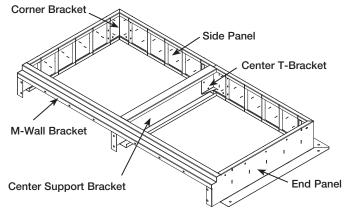
\*Image shown is a representative drawing. Actual curb for bypass air plenum section may have additional pieces, depending on quantity of fans. Image is for a two fan system.
