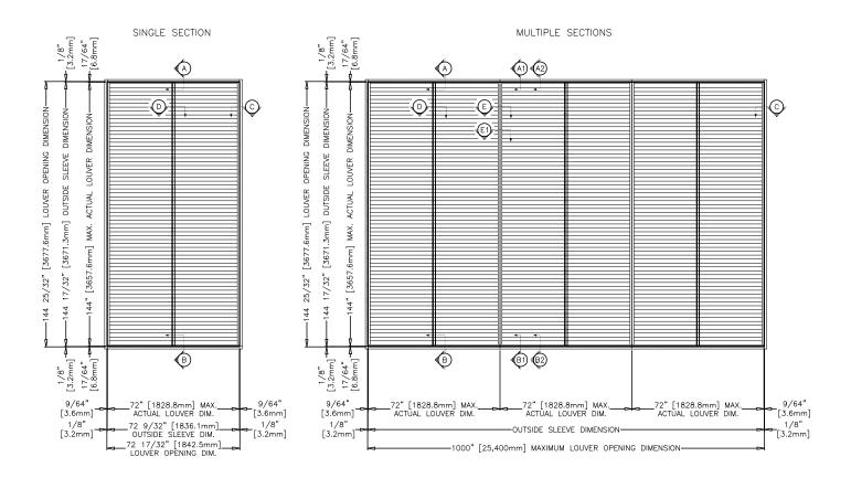
Minimum Rough Opening Size 12 in. W x 12 in. H Maximum Single Section Rough Opening Size 72.50 in. W x 144.50 in. H
