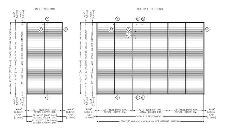
Minimum Rough Opening Size 12 in. W x 7 in. H Maximum Single Section Rough Opening Size 72.50 in. W x 144.50 in. H
