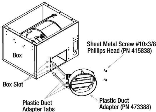
**2** Rotate plastic duct adapter (PN 473388) until the screw tabs meet the box.
