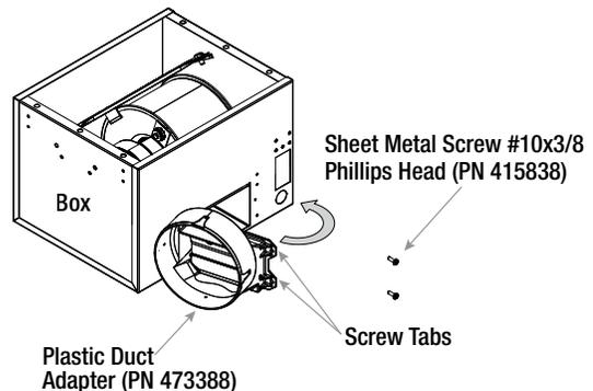
**3** Install screws provided to secure discharge.
