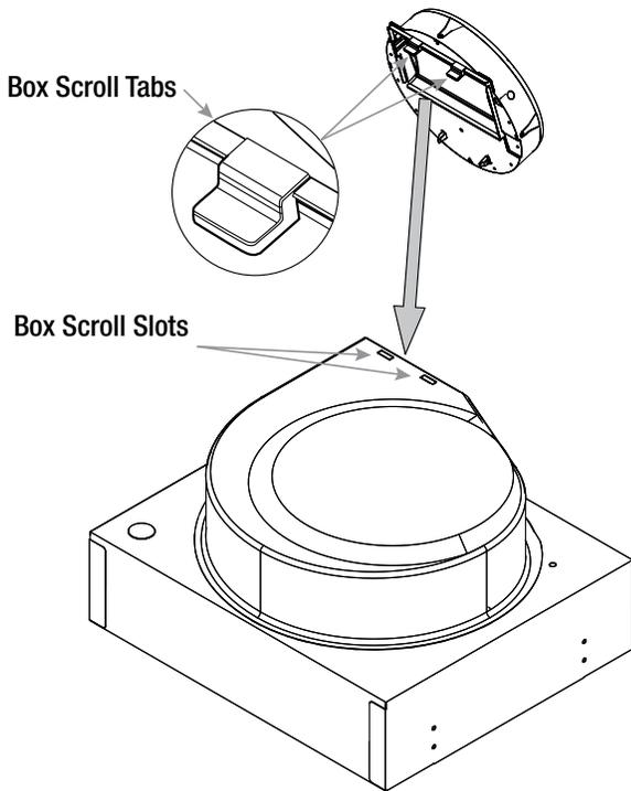
**2** Rotate plastic duct adapter (PN 474433) until the two mounting tabs fully engage into the two box mounting slots.
