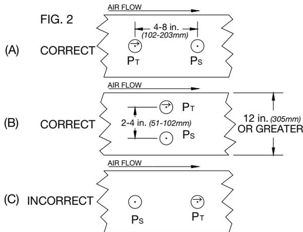
Connect the total pressure probe to the "H" port of the control/transducer and the static pressure probe to the "L" port.
