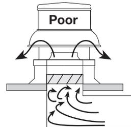
Dampers must open fully. Use motorized dampers in low airflow applications to reduce losses.
