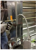
2. Disconnect the conduit from the sleeve.
