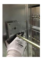
16. Re-assemble the RRL (or RRL/OCI, TOR) assembly. Mark the holes on the frame where you are going to mount the bracket. Drill and attach the bracket.
