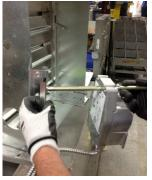
14. Re-assemble the RRL (or RRL/OCI, TOR) assembly. Mark the holes on the frame where you are going to mount the bracket. Drill and attach the bracket.
