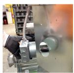
9. Loosen the bolts on the right side that holds the jackshaft bracket. Remove the jackshaft bracket on the left side. Loosen the bolts on the right side that holds the jackshaft bracket.
