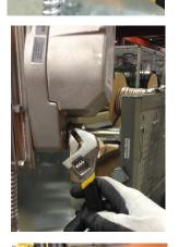
Take junction box with RRL (or RRL/OCI, TOR) and rubber gasket off of the sleeve.
