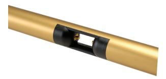
The nodes in Vari-Green probes utilize a highly engineered injection molded aperture that straightens the airflow as it passes over the thermistors to produce an accurate measurement.
