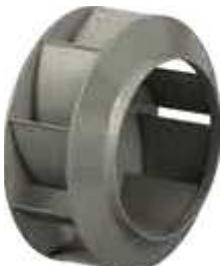
Greenheck BCSW-FRP centrifugal fans have non-overloading backward curved blades. Every wheel is laid up by hand. The blades are strapped to the backplate rather than just glued to ensure a stronger wheel. The backplate
