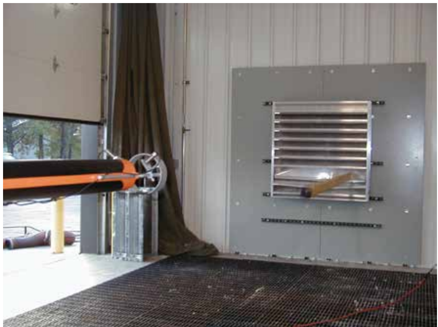
Greenheck's onsite missile impact test
