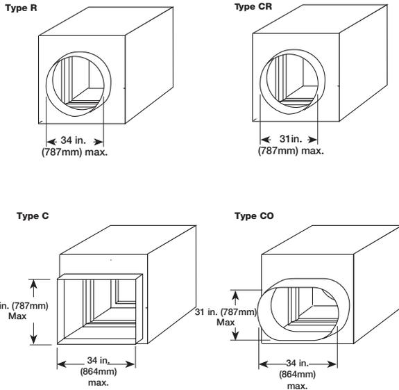
C, CO, CR transitions are positioned 1 in. (25mm) from bottom of sleeve.
