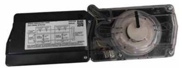
Smoke detector requires 100 fpm minimum air velocity in duct. For damper activation requirements when system velocity is less than 100 fpm, the local authority having jurisdiction should be consulted.
