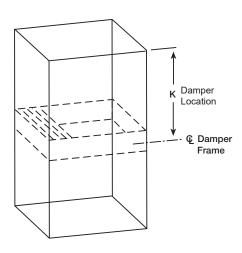
Note: Horizontal dampers must be installed with the "K" dimension on the top side as shown (per UL test: see label on damper). Horizontal dampers must have the access door installed on the top side to facilitate re-opening of the blades should the link melt.
