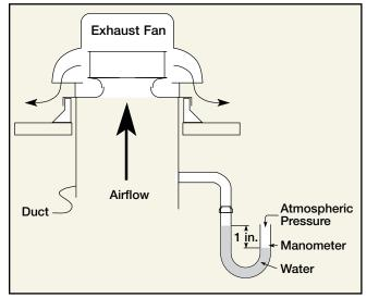
To calculate the system losses, one must know the ductwork system configuration (see Ductwork figure).
