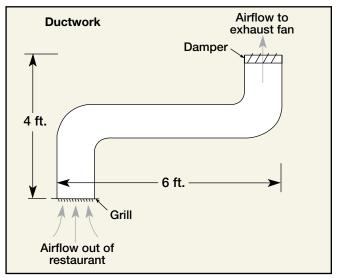
There is also a 0.08 in. pressure drop for each resistive element or fitting. For this example, there are 5 fittings: one grill, two duct turns, one damper and louver in the wall of the office. The total pressure drop for fittings is:
