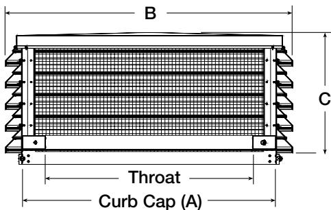
Greenheck designs penthouse units for use in gravity intake or relief applications where aesthetics are important.
