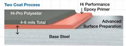
LabCoat corrosion-resistant coating is electrostatically applied uniformly in two steps that bond the coating to the properly cleaned and prepared metal surface.
