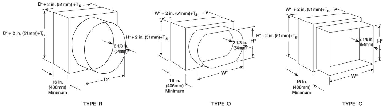
\*These dimensions are furnished approximately 1/4 in. (6mm) undersize, except round and oval dimensions which are approximately 1/8 in. (3mm) undersize.
