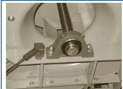
A tri-axial accelerometer measures the velocity amplitude in the horizontal, vertical, and axial directions.
