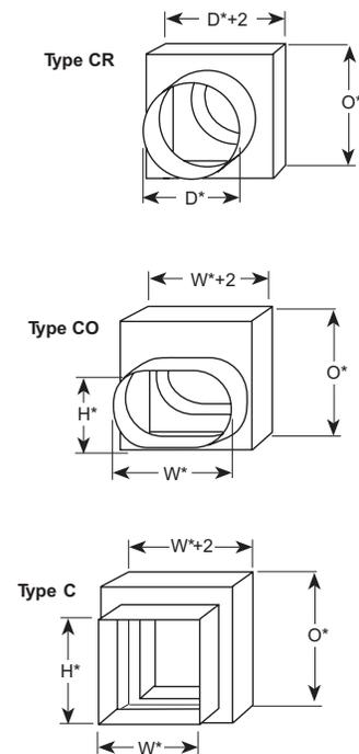
C, CO, CR transitions are positioned 1 in. (25mm) from bottom of sleeve.
