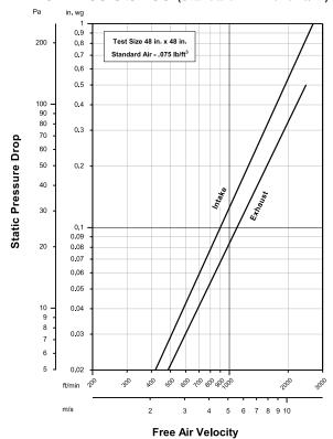
Model ESU-154 resistance to airflow (pressure drop) varies depending on louver application (air intake or air exhaust). Free area velocities (shown) are higher than average velocity through the overall louver size. See louver selection information.
