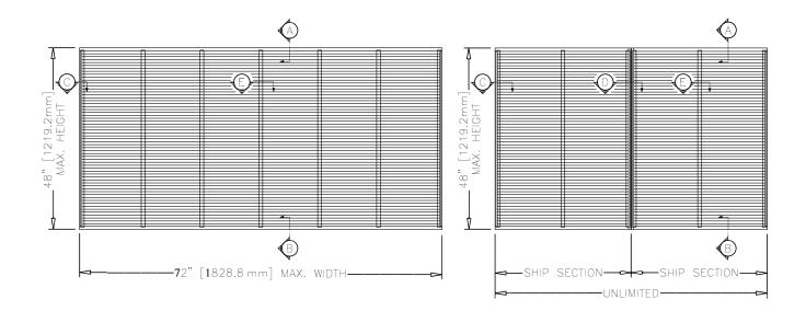
Minimum Single Section Size 13 ½ in. W x 10 in. H (without flange) 13 ½ in. W x 12 in. H (with flange) Maximum Single Section Size 72 in. W x 48 in. H
