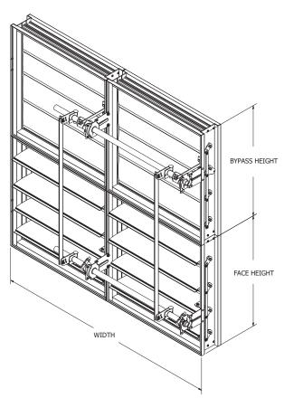
Note: If units are over 84 in. (2159mm) high, the face and bypass damper will ship separately and require field assembly.
