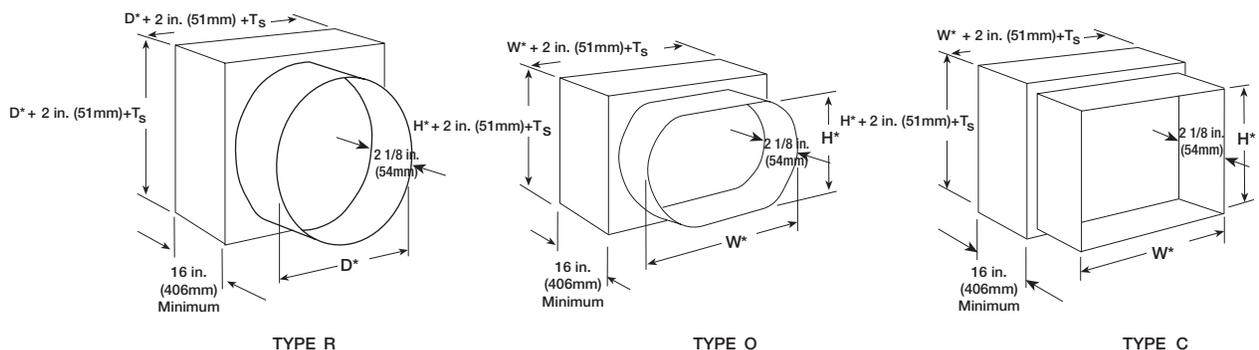
\* These dimension are furnished approximately 1/4 in. (6mm) undersize, except round and oval dimensions which are approximately 1/8 in. (3mm) undersize.
