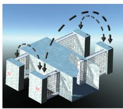
\* The Greenheck model IDHE-O duct heater is universally configured to allow airflow in either direction in all mounting orientations.
