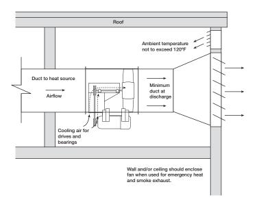
For the greatest amount of internal cooling, discharge static pressure should be kept to a minimum while keeping most of the pressure on the inlet side. Locate the fan at ends of the duct runs and near the discharge point in the system. This setup will promote the ambient air cooling effect.
