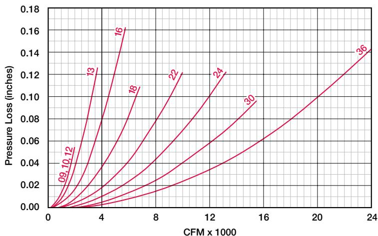
TCBRS fan selections can be made using the TCB inline performance data (pgs. 12 to 31) along with the following system effect curves. The pressure loss (determined from information in the System Effect Curve to the left), must be added to the external system static pressure to ensure accurate selections. Greenheck's computer aided product selection CAPS® software will add these system effects automatically.
