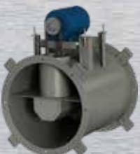
Model TCB centrifugal backward-inclined belt drive fans are for higher pressures. Capacities range from 300 cfm (500 m<sup>3</sup>/hr) to 26,000 cfm (44,200 m<sup>3</sup>/hr) and up to 4 in. wg (1000 Pa) of static pressure. Maximum operating temperature is 200°F (93°C). Model TCB is available with UL 762 for restaurant exhaust.
