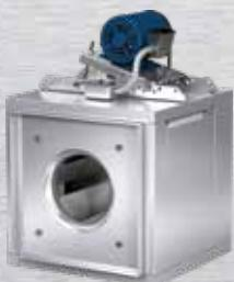
Models SQ and BSQ centrifugal backward-inclined belt or direct drive fans are for clean air applications (intake, exhaust, return, or make-up air systems) where space is a prime consideration. Capacities range from 60 cfm (102 m<sup>3</sup>/hr) to 27,000 cfm (45,870 m<sup>3</sup>/hr) and up to 4 in. wg (1000 Pa) of static pressure. Maximum operating temperature is 180°F (82°C).
