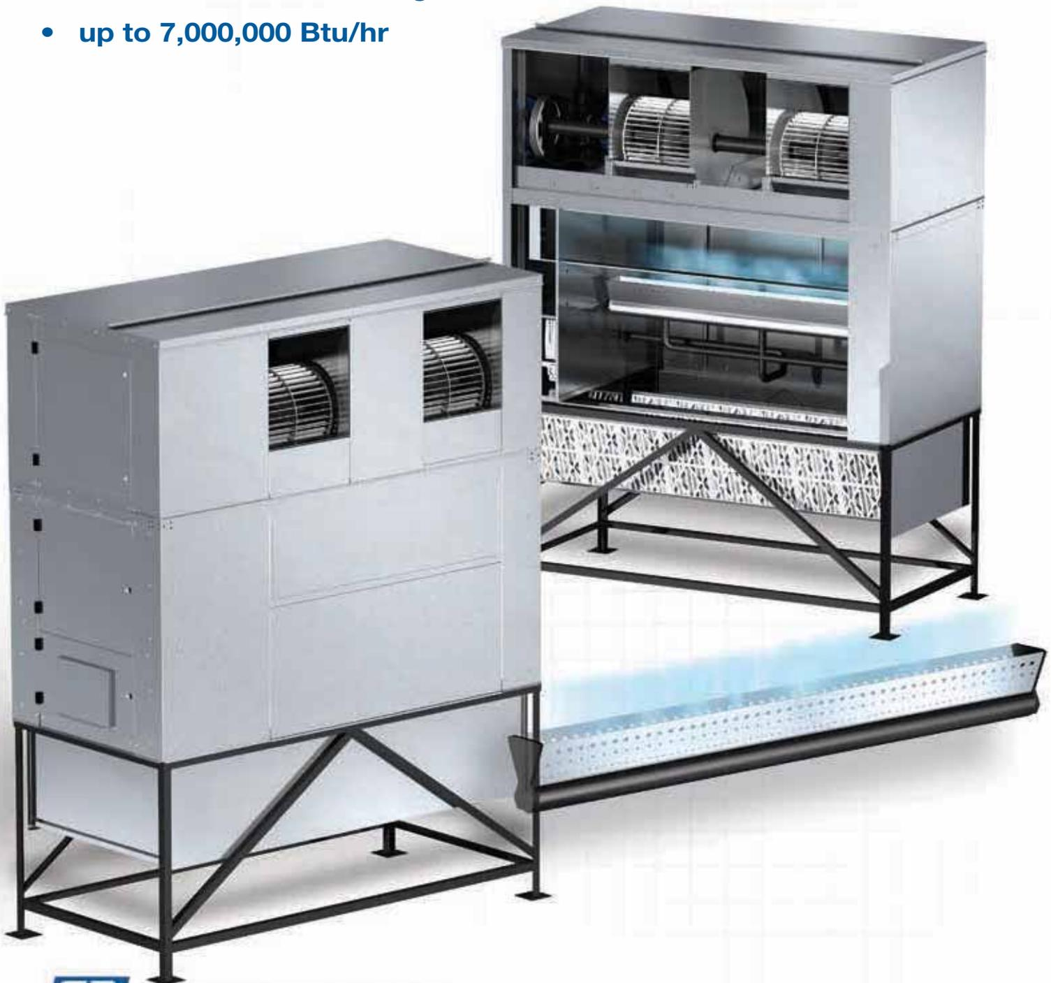
The Greenheck model VSU uses direct gas-fired technology to provide efficient ventilation and heating in any climate. A 92% thermal efficient line burner reduces gas consumption for maximum energy savings for both natural gas and propane fuel sources. The vertical configuration removes the equipment weight load from the roof and offers an easier means of installation. Ground level filters, dampers, and controls also greatly simplify equipment start-up and maintenance.
