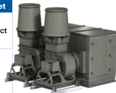
C Series - Exhaust fan with scroll housing and non-overloading centrifugal wheel. Fans mount next to the energy recovery plenum.
