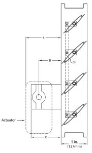
This drawing depicts the worse case clearance requirements for an actuator with a jackshaft.
