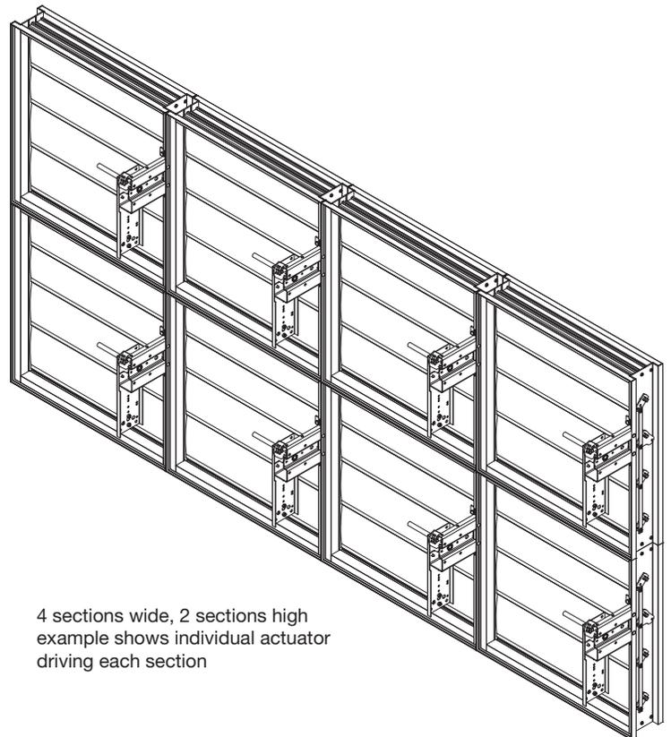
4 sections wide, 2 sections high example shows individual actuator driving each section
