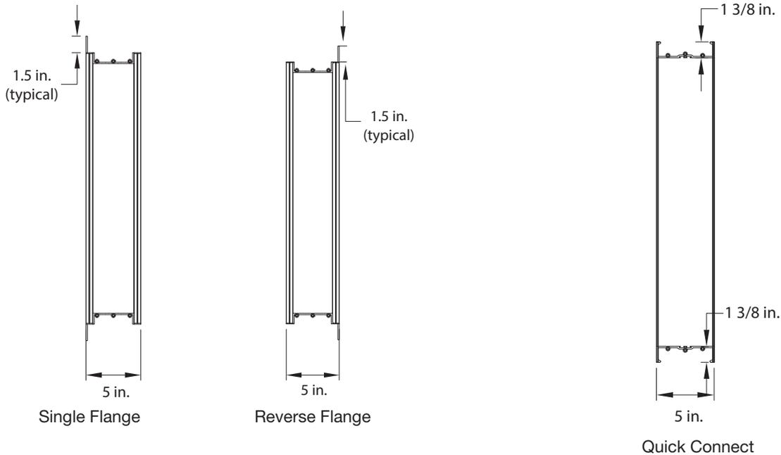
\* Width and height is based on outside dimension. W & H dimensions furnished approximately 1/4 in. (6mm) undersize.
