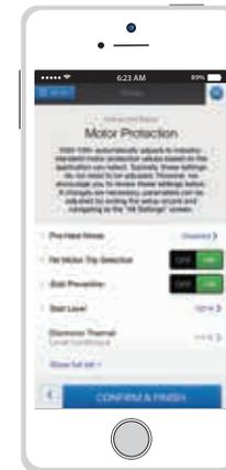
9. Optional: Review and adjust the motor protection settings. These are factory defaulted to industry standards. Tap "Confirm & Finish".
