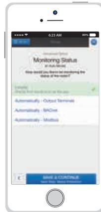
8. Select how you wish to monitor the Vari-Green Drive/fan. If anything other than locally, configure the inputs/outputs and verify the appropriate wiring connections. Tap "Save & Continue".
