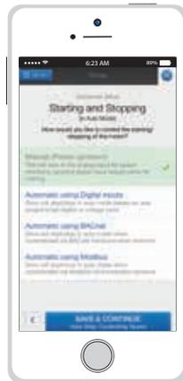
7. Select how you wish to start/stop the fan. If anything other than manual, configure the inputs/outputs and verify all additional wiring connections. Tap "Save & Continue".
