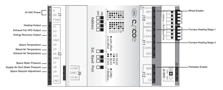
The expansion board is an I/O module than can be used to monitor additional statuses or provide commands from medium board controller.
