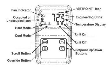
Override Button Function - The display shows a person in the lower left corner of the display at all times. If the person is solid, the unit is operating in occupied mode. If it is an outline of the person, the unit is in unoccupied mode. Pushing the Override button when the unit is in unoccupied mode will allow a temporary override sequence to Occupied mode for a period of 1 to 3 hours (adjustable at the unit microprocessor).
