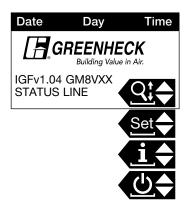
THE INITIAL MENU SCREEN DISPLAYS THE PROGRAM VERSION, CONFIGURATION CODE AND STATUS LINE. THE STATUS LINE DISPLAYS WHICH MODE THE FURNACE IS IN.
