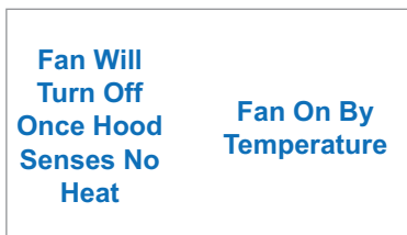
Example of screen as user attempted to shut off fan while fan is above cooking detection temperature setpoint.
