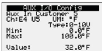
**Viewing c.pCOe Auxiliary Values** - Once the expansion board I/O is configured, the user can view and/or change the I/O type by navigating to Ctrl Variables/Aux I/O Config.
