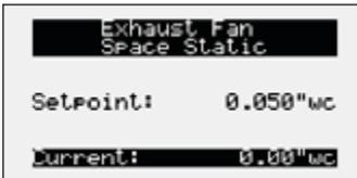
**Space Pressure** – Fan speed is determined by building pressure control loop.
