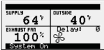
THE INITIAL MENU SCREEN DISPLAYS THE JOB NAME, UNIT TAG, UNIT STATUS, OUTSIDE AIR CONDITIONS, SPACE CONDITIONS AND SETPOINTS.
