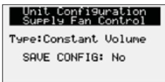
THIS SCREEN ALLOWS THE USER TO VIEW AND CHANGE THE SUPPLY FAN CONTROL TYPE.
