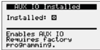
**Enabling the c.pCOe in the Main Controller.** - To enable the c.pCOe expansion I/O module, go to Ctrl Variables/Advanced/Unit Config. User will have to enter the Service Password to make any edits at this point. Consult factory for configuring the expansion board. The expansion board must be enabled to configure spare I/O points. Once enabled, the user must reboot the controller. See screens to the left for expansion board enable points.
