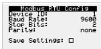
THIS SCREEN ALLOWS THE USER TO ADJUST MODBUS PARAMETERS.
