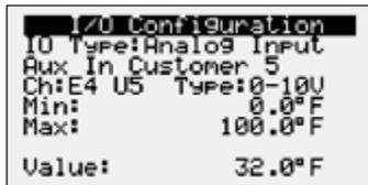
**Change or Update the I/O Point** - Once the editable option is selected, the user must scroll to the I/O Configuration Menu. At this menu the desired I/O type can be selected. Once selected the user can configure the desired channel at the expansion board. The channel will have an 'E' designation for expansion board. Aux In Customer 1-10, Aux Analog Out 1-4, and Aux Digital Out 1-6 will be allocated for the I/O expansion board. See example to the left.
