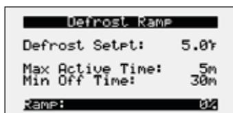
THIS SCREEN DISPLAYS THE TEMPERATURE AT WHICH THE UNIT WILL ENABLE FROST CONTROL MODE IF NECESSARY (FACTORY DEFAULT=5°F)
