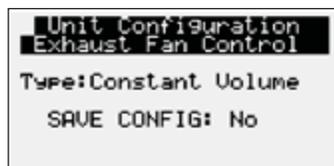
THIS SCREEN ALLOWS THE USER TO VIEW AND CHANGE THE EXHAUST FAN CONTROL
