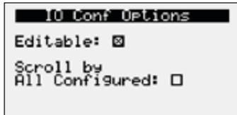
**Configuring the I/O Type** - In order to edit and configure the I/O configuration of the unit, go to Ctrl Variables/Advanced/I/O Configuration. The user must enable the Editable option for configuring I/O points. If configuring a new I/O point, 'Scroll by All Configured' must be deselected to view all I/O options.
