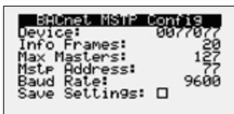
THIS SCREEN ALLOWS THE USER TO ADJUST BACNET AND MSTP PARAMETERS.
