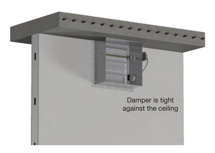
Perfect for installations where the damper sleeve is tight up against a wall, floor, or other obstruction. This UL approved installation method allows retaining angles to be installed on only three sides of the damper. The fourth side can be attached directly to the opening without the need for an angle or any firestop material.
