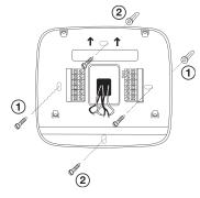
For vertical mount put one screw on the top and one screw on the bottom.
