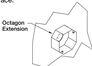
4. Insert the compression seal into the hole from the inside of the hood making sure the gasket is placed on the fitting before inserting it into the hole. Place the octagon box and J-box plate provided over the fitting on the top of the hood, keeping the fitting centered in the box. Install the lock washer and 1-1/2 inch (38.1 mm) nut on the threaded portion of the compression seal and tighten securely.
