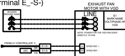
**VFD Provided by Others, Control Wiring - if equipped**
