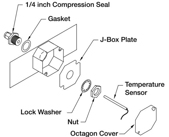
5. Insert the temperature sensor into compression seal and tighten to 35 ft-lbs (47.5 Nm).
