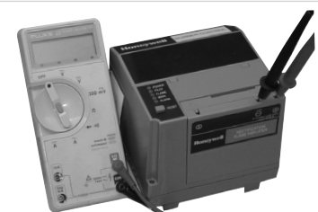
Fig. 4 DC Voltmeter and Flame Amplifier
