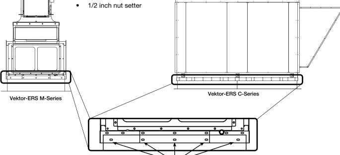
Install supplied bolts through BAP skirting into roof curb.
