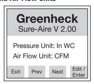
**Pressure Units:** Press "Edit" to change pressure units. Press "Prev" or "Next" to adjust, then press "Enter" to store the value.
