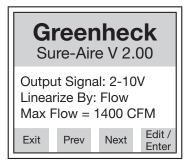
**Output Signal:** Press "Edit" to change Output Signal type. Press "Prev" or "Next" to adjust, then press "Enter" to store the value.
