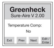
Press "Edit" to change Temperature Compensation. Press "Prev" or "Next" to adjust, then press "Enter" to store the value.
