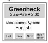
Press "Edit" to change the measurement system units. Press "Prev" or "Next" to adjust, then press "Enter" to store the value.
