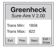
**Transmitter Min Value:** Press "Edit" to change Transmitter Min Value. Press "Inc" or "Dec" to adjust, then press "Enter" to store the value.
