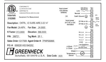
Match the Tag Mark on the Sure-Aire electronics tag to the Tag Mark on the fan nameplate. Sure-Aire electronics are supplied set-up individually for a specific model and performance. Contact factory if Sure-Aire electronics are being used on a different Tag Mark then specified.
