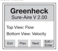
**Top View:** Press "Edit" to change Main Display Value. Press "Prev" or "Next" to adjust what reading displays on the Home screen, then press "Enter" to store the value.
