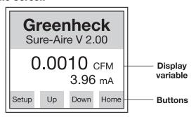
To view display variables, use the "Up" and "Down" buttons to scroll through the list. To adjust parameters, press "Setup" and scroll through the settings.
