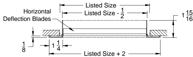
Model: XG-H4002-1 Single Deflection Grille - Horizontal Blades
