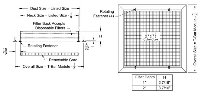
Note: This product complies with NFPA 90A-18 standard 4.3.7.3.2 and 4.3.8.3.2 and is constructed with openings through which a 1/2" sphere can not pass.
