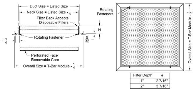
Note: This product complies with NFPA 90A-18 standard 4.3.7.3.2 and 4.3.8.3.2 and is constructed with openings through which a 1/2" sphere can not pass.
