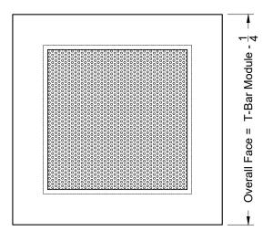
Note: This product complies with NFPA 90A-18 standard 4.3.7.3.2 and 4.3.8.3.2 and is constructed with openings through which a 1/2" sphere can not pass.
