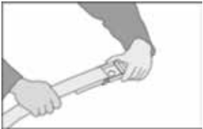
Fig. 2 Hook the ends through the slots in the bracket.
