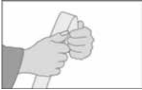
Fig. 1 Both ends of the strip are bent over 8-10 cm. Protect your hands with gloves.
