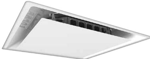
Models XG-5700 / XG-5700A 2 Cone diffusers are designed to efficiently handle cooling temperature differentials of 18-20°F at ceiling heights of 8' to 10'. The round neck to square face design provides a uniform 360° fixed horizontal air diffusion pattern. For applications requiring a vertical air flow, the XG-5700A adjustable model employs movable air deflecting vanes which will provide vertical downward airflow.
