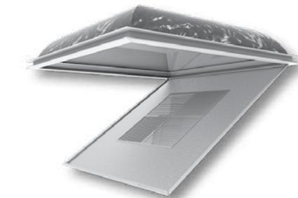
Air Outlets shall be aluminum face model XG-7350 or steel face model XG-7350 AF manufactured by GREENHECK. Units shall consist of 51% free area perforated face fixed to a formed fiberglass backpan. Perforated holes shall be 3/16" diameter on 1/4" staggered centers. Exposed fiberglass backpan shall have an aluminum foil liner. The outlet's backpan shall be factory scored to allow field installation of a tab lock collar or spin-in fittings
