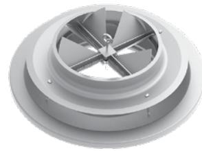
Pattern adjustment operator shall open the inner opposed blade damper assembly to discharge the air in a vertical pattern or close the damper to allow a tight horizontal pattern. In the horizontal setting, core shall project discharge pattern to minimize ceiling smudging. The inner core assembly shall be removable for installation and for access into the ductwork.
