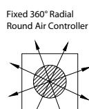
Air Deflection Patterns Obtained By Adjusting Air Pattern Controllers
