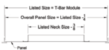
Model: XG-4002R-6 (Ceiling Return Grille - Lay In T-Bar) (V-Vertical Or H-Horizontal Fixed Blades)
