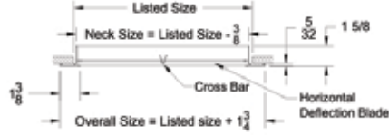
Model: XG-H4002R-1 (Sidewall Return Grille - Surface Mount) (Horizontal Fixed Blades)
