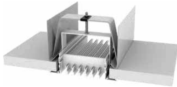
Hanger Bracket Install – Hemmed Plenum
