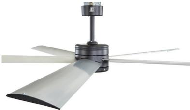
Aluminum airfoils are designed to maximize airflow, boost efficiency, and optimize coverage area. Airfoils are available in mill, powder-coat, woodgrain, or anodized finishes. Winglets are designed to reduce fan noise.
